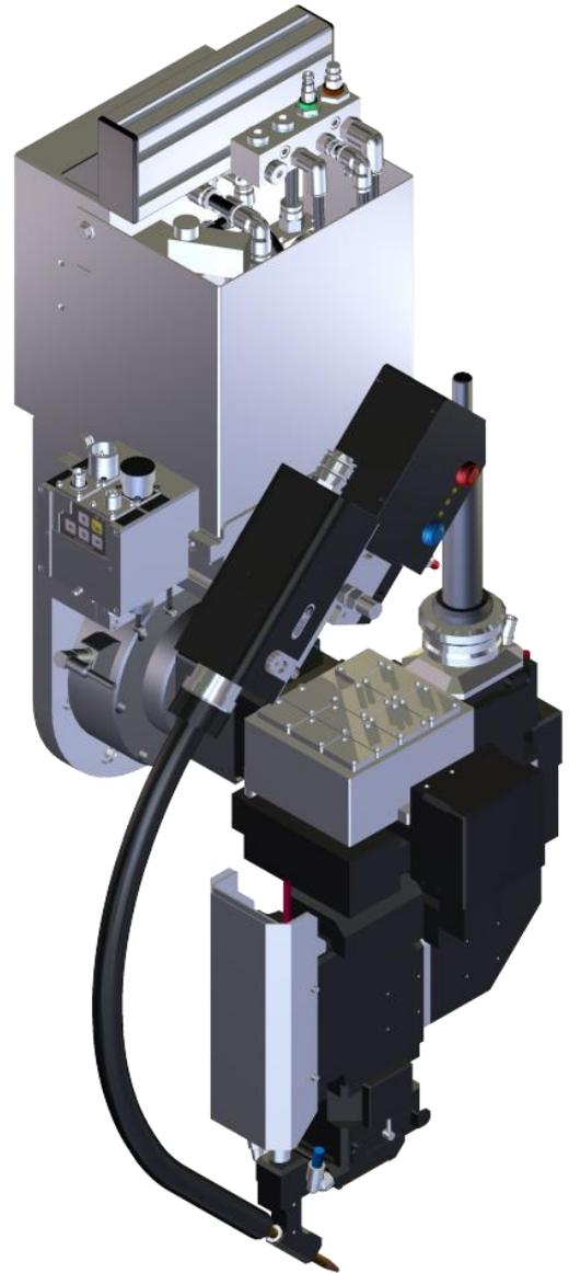
An application example: ALO3 with the wire-feed module and GAS media coupling
