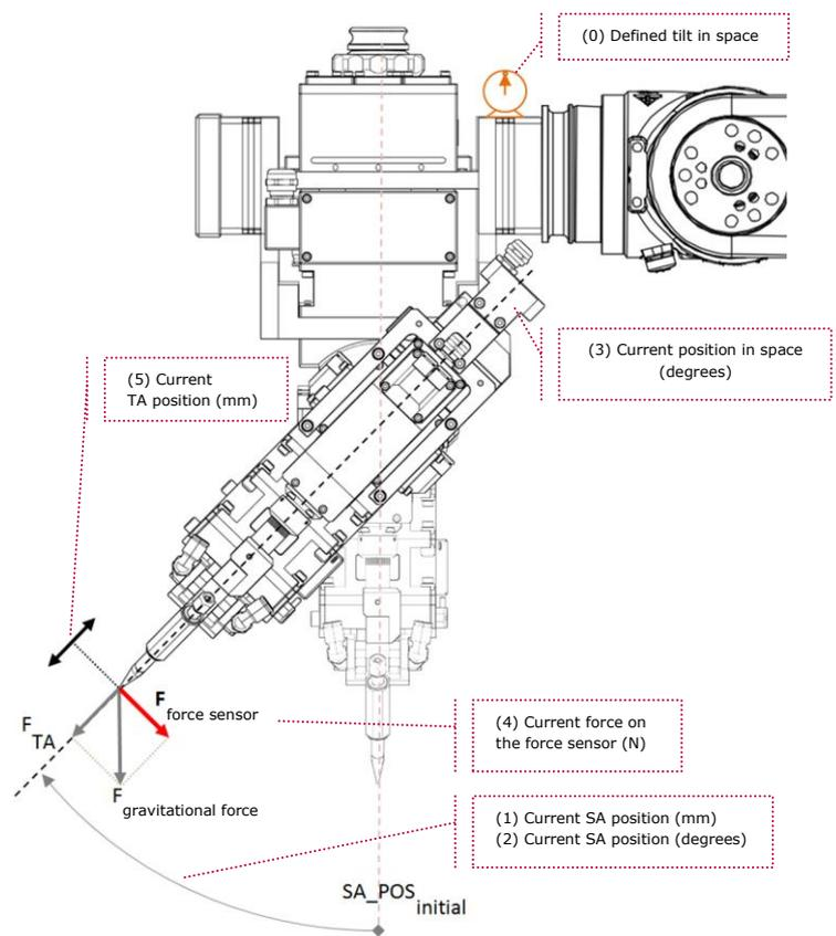
Figure 2: Measuring signals from the ALO3 processing unit
