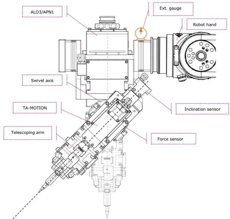
Figure 1: Actuator/sensor modules on the ALO3 processing unit
