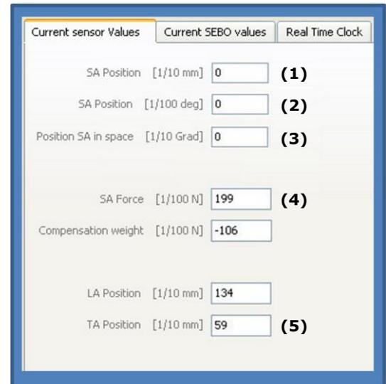
Figure 3: Sensor measurements in the Basis HMI-B parameterization software
