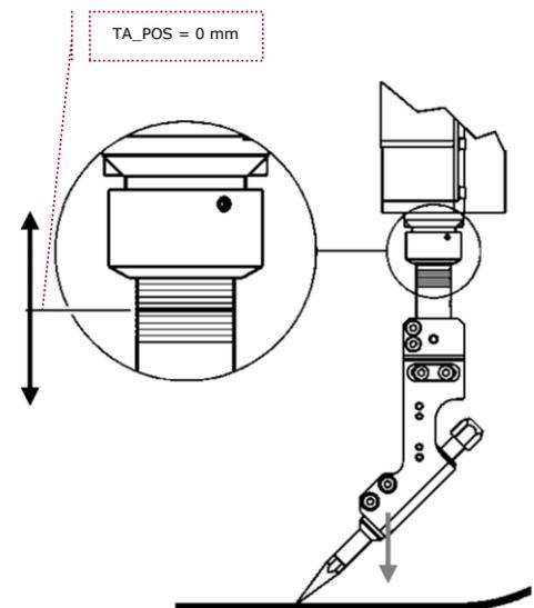
Figure 4: Immersion depth of the telescoping arm
